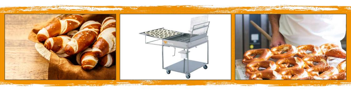
The manual lye application unit Tauchboy offers an easy and manual way of lying small quantities. Due to the compact design it can be used in small production or directly in the store. It enables to apply lye on up to 800 dough pieces daily.
